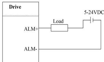
**Figure 6** Sinking output
